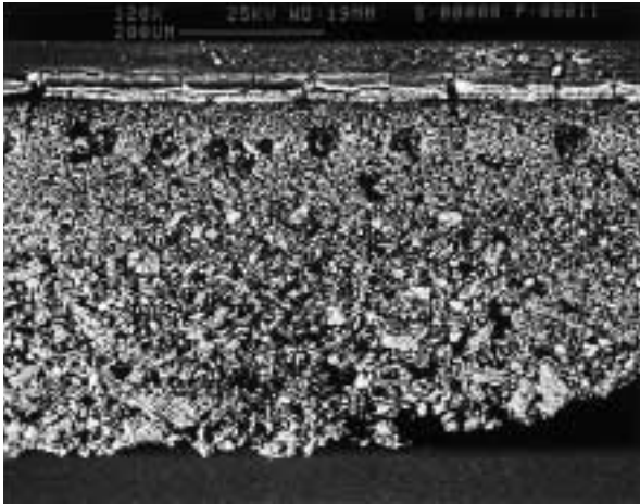
FIG. 2 Cross-section of paint and gesso ground as a back-scattered electron image in the scanning electron microscope, showing coarse gesso and finer gesso at the surface beneath the paint layers. Original magnification 120X; actual magnification 88X.
